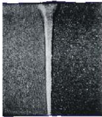
Beam welding Plain butt weld 30 mm Almost no shrinkage
