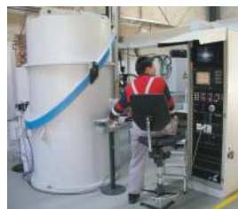
Electron beam welding of conveying belts 0.2 mm
