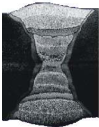
Inert gas welding Double V-weld 30 mm Strong shrinkage
