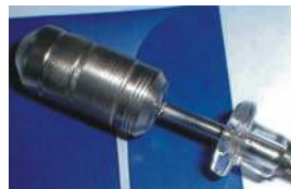
Electron beam welded tungsten anode
