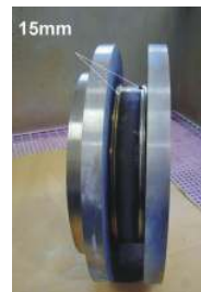
Rundnaht DN 300, 15mm tief, 15Mo3
