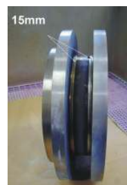
Rundnaht DN 300, 15mm tief, 15Mo3
